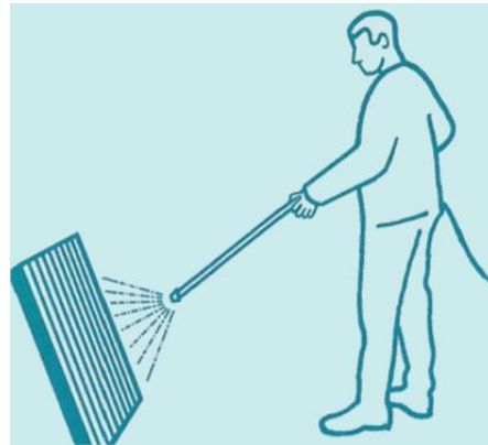
Clean the mat with a high-pressure cleaner, a garden hose or a hard scrubbing brush in combination with water and a universal detergent.
